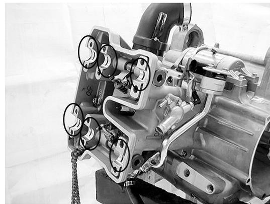
Install the cam chain over the cam sprockets and then install the intake and exhaust camshafts.
